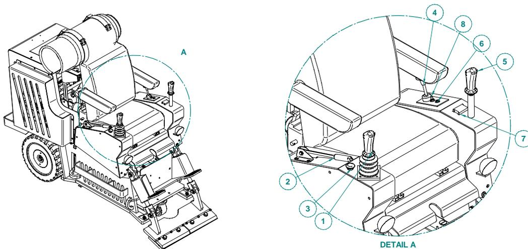
1. Steering is controlled by means of two independently driven wheels. The driving speed is controlled by the movement of the motion control joystick.
