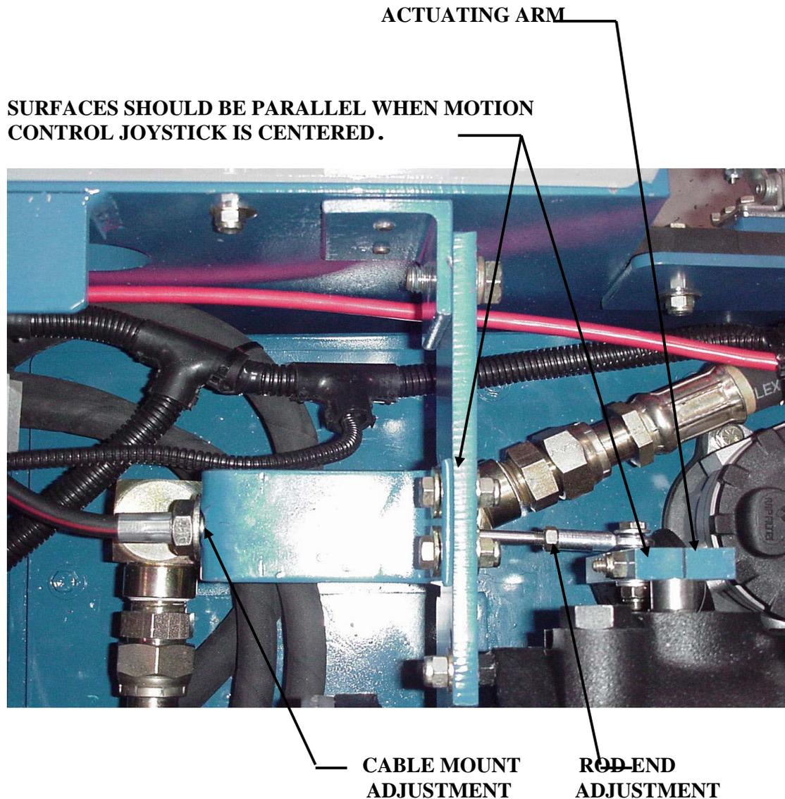
Note: The position of the cable rod end may be adjusted at the cable mount and at the rod end of the cable. Make sure that the actuating arm is straight up and down when the motion control joystick is centered.
